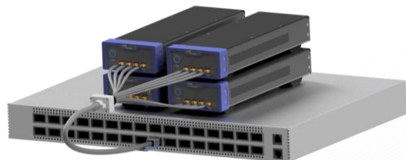
Figure 3 Switch Testing using 4 Pulsars.
